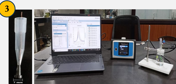
An electrode assembly for electrochemical biosensing of heavy metals and a process for the preparation thereof. (by Ankur Singh, PhD Research Scholar and Prof. Vipin Kumar) (Indian Patent No.202231076821 dated 29.12.2022)
